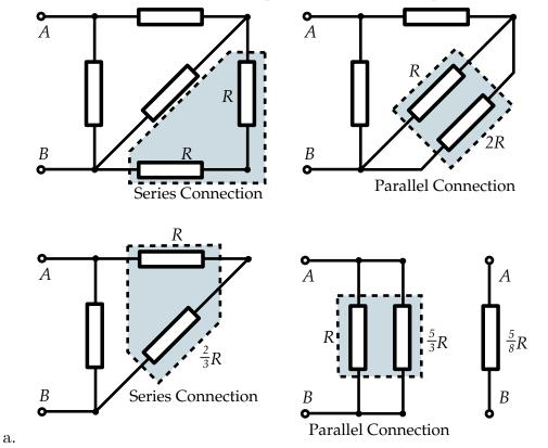
4. The circuit with all resistors of equal resistance, R, simplified:
