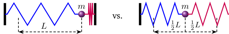
Figure 3: The spring-sandwich: In the initial position at left, the left-hand side spring is at its equilibrium length, L , while the right-hand side spring (physically identical to the left-hand side one) is maximally compressed. In the position at right, both springs are compressed to half of their equilibrium length.
